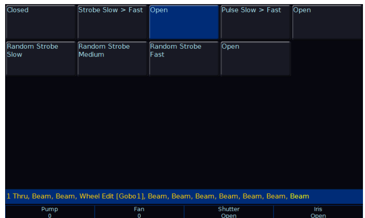
Example of the display after the central encoder button has been pressed on a “shutter” parameter. The highlighted value (in blue) shows the currently active value.
