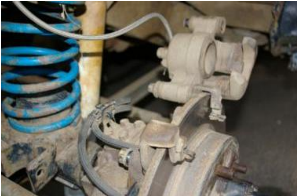
Figure 7. Both lock and unlock tubes (black braided tubes) - the unlock tube is the lower tube that comes down to the front of the hub.
