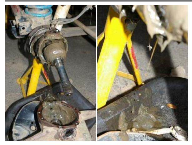
That's water pouring out of the axle! Below is a worn out bearing.
