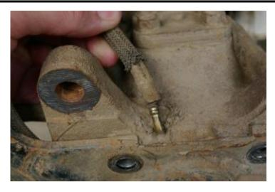
Using a splitter, split the steering joints (two to do on the passenger side and one on the driver - UK)
