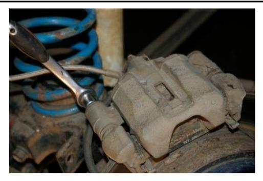
The caliper then opens up using the rear bolt as a hinge.
