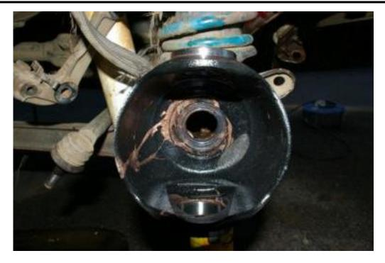
Pack the CV with grease (but do not overpack) and re-fit the driveshaft.
