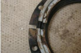
Tighten the seal bolts to 7.5 ft/lbs.
