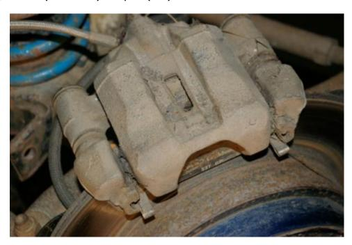
Using a 12mm spanner, release the front caliper bolt (the left is the front of the car in this picture) and loosen the same bolt on the rear of the caliper.
