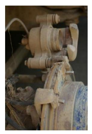
The pads are retained by small spring clips, a simple pull on the pads (horizontally away from the disk) should remove them (or gently prise out the pads with a small screwdriver - do not remove the spring clips)
