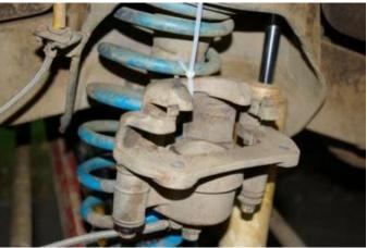
Now the front brake disc can be removed. If you are lucky it will simply pull off but if you have problems then there are two M8 holes in the disk hub. Simply run two bolts into these holes and the disk will push off the hub. The picture below shows a bolt being used to push the disk off the hub.
