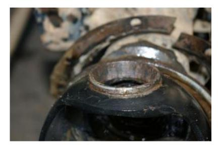
These can be really difficult to drive out but I found a simple way forward. I used my welder and welded a small blob of metal to the inside of the ring. This then created a rough part that a screwdriver or chisel can get a purchase on and then using a hammer it can be easily driven out.
