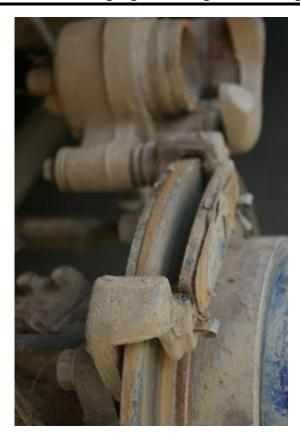
The caliper is held on with two bolts at the rear (see below). Release the bolts and tie the caliper to the spring to keep it out of the way.
