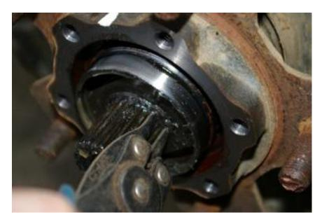
Remove the bolts holding the disc backing plate (and the hub) to the knuckle joint.
