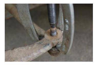
At the rear of the hub release the small bolts holding the seal and retainer. You can see that the swivel hub is covered in oil, a bad sign for KingPin problems.
