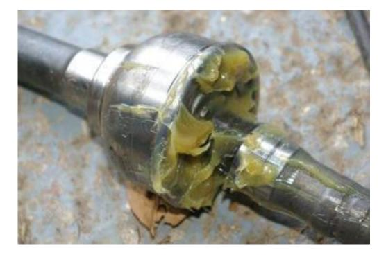
Grease the new KingPin bearings and insert the top one in the carrier.
