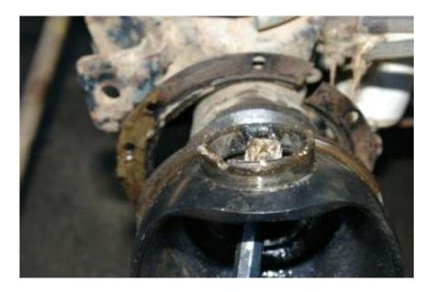
The new rings can then be driven into place with a piece of wood to protect them from the hammer. I also hooked out the small axle shaft oil seal and put a new one in, again these can be obtained from most bearing dealers, they are  $26 \times 38 \times 7$  R23/TC specification. If you are rich you can get the Suzuki parts instead - 09283-26016,
